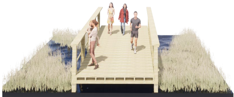
Figure 32 - Typical Section for a boardwalk over wetlands
