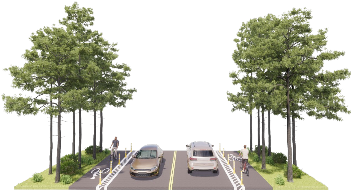
Figure 35 - Typical section showing roadway shoulders converted to separated bike lanes with a buffer to improve safety for cyclists
