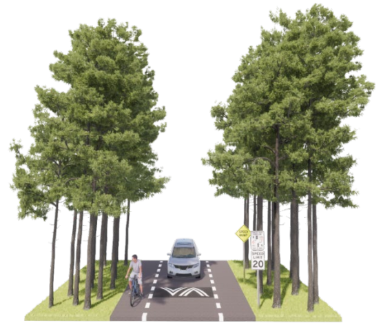
Figure 37 - Typical Section for an Advisory Bike Lane where pavement width is not adequate to stripe out separated uses for both cars and bikes
