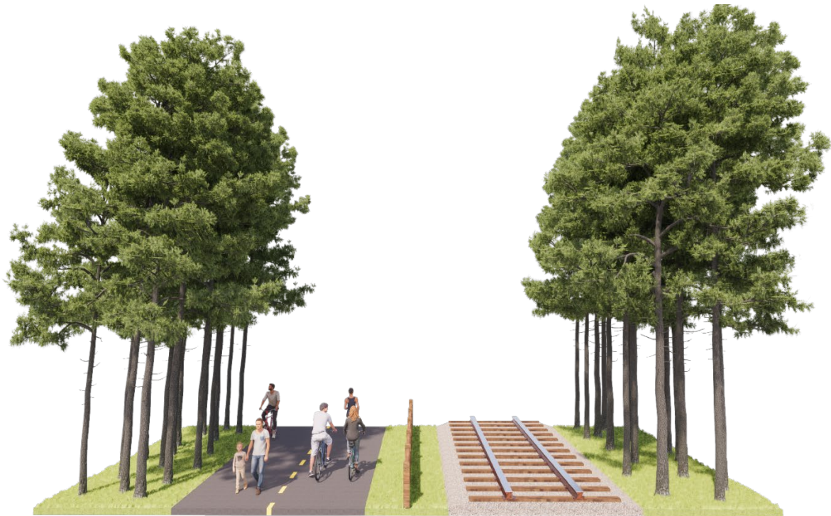
Figure 31 - Typical Section for a trail along a railroad
